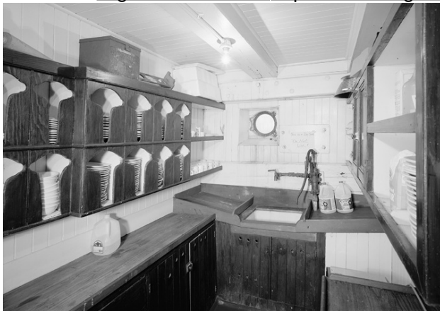
Figure 4.5. The Steward's stores and pantry on steam schooner Wapama . This shows another variation on the shelf design, to keep dishes from falling out and breaking at sea. Reproduction Number: HAER CAL,21-SAUS,1—16 in Collection: Historic American Buildings Survey/Historic American Engineering Record/Historic American Landscapes Survey . Courtesy of Library of Congress Digital Collections. http://www.loc.gov/pictures/item/ca1521.photos.013124p/ .
